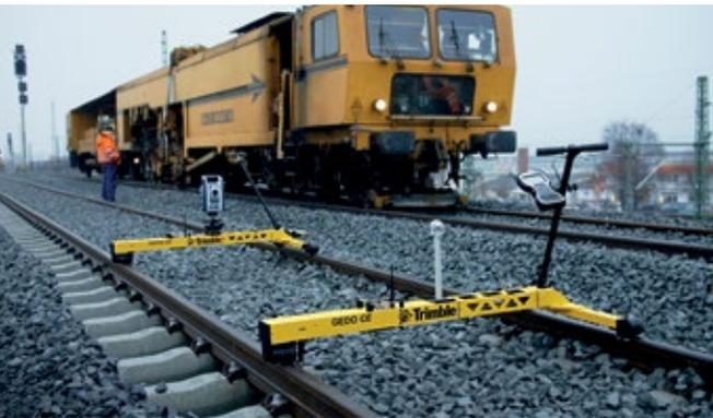
Tamping is essential for railway maintenance to ensure track quality and stable ballast. Trimble GEDO provides an integrated solution for measurement and quality control to support tamping machines and operations.
