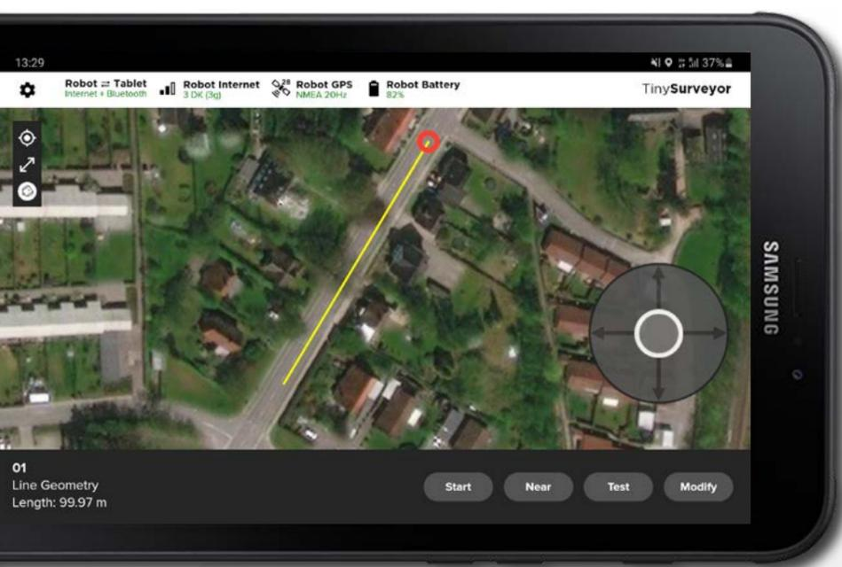
The accompanying tablet gives the operator full control of the robot as well as the parameters of the job in question. For instance, the operator can customize marking settings, apply projection shifts and adjust robot velocities directly from the tablet. Existing CSV and DXF files can be sent directly from the tablet to the TinySurveyor, allowing operators to start working minutes after arriving on site.
